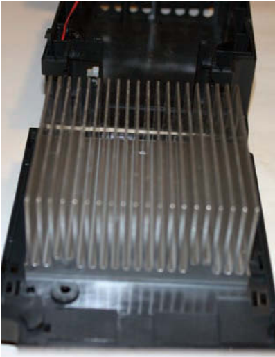
Figure 6 The Altivar 12 heat-sink assembly for the Infineon Easy PIM module mechanically connects on the flat rear surface of the heat sink and thermally connects with thermal grease.
