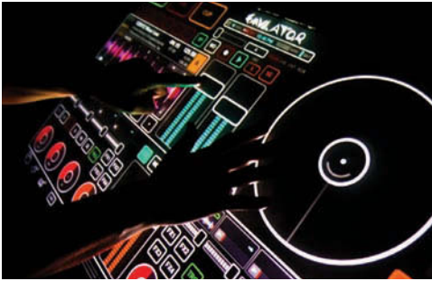
Figure 3 The SmithsonianMartin Emulator DVS DJ System is a transparent mixing desk that allows the audience to see the DJ through the mixing panel. Cameras in the corners can track finger movement, enabling the display.
