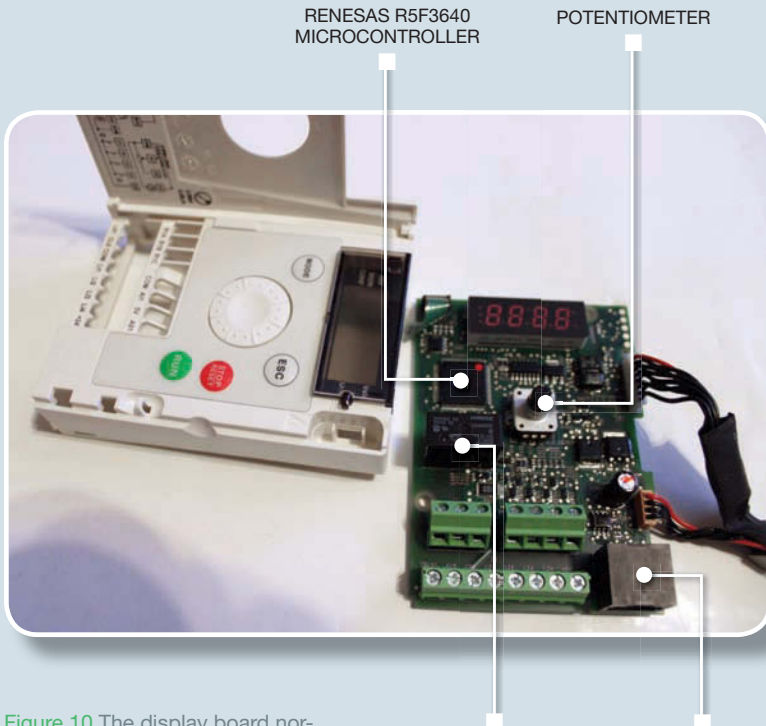
Figure 10 The display board normally resides behind the front panel, and a Renesas microcontroller drives and controls the display and the Modbus-serial-port connection.
