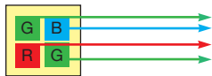
Figure 4 The four-chip LED products containing RGGB (red/green/green/blue) are typically for one-channel illumination.
